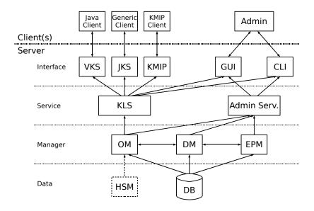
Figure 1: Key-Lifecycle Management System architecture (see text).
